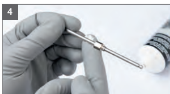
4 Grease paint needle around the needle packing area
