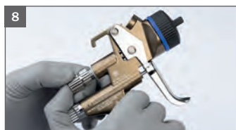
8 Install material flow control screw
