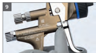
9 Grease visible part of air piston rod
