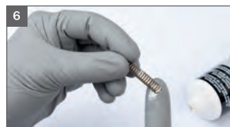
6 Grease and insert paint needle spring
